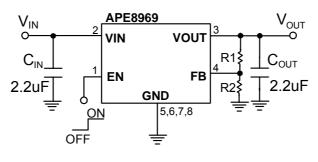
$V_{OUT}=V_{FB} x (1+R1/R2), V_{FB}=0.8V$ R2 range = 50K~300K
