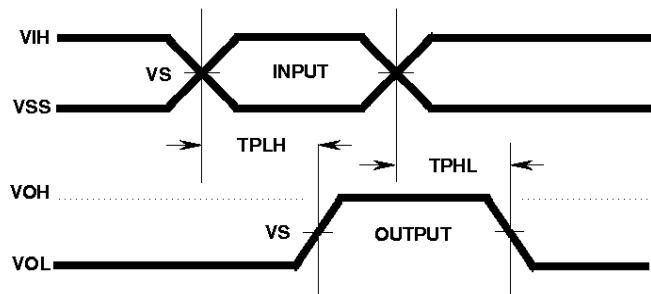
***Propagation Delay Load Circuit***
