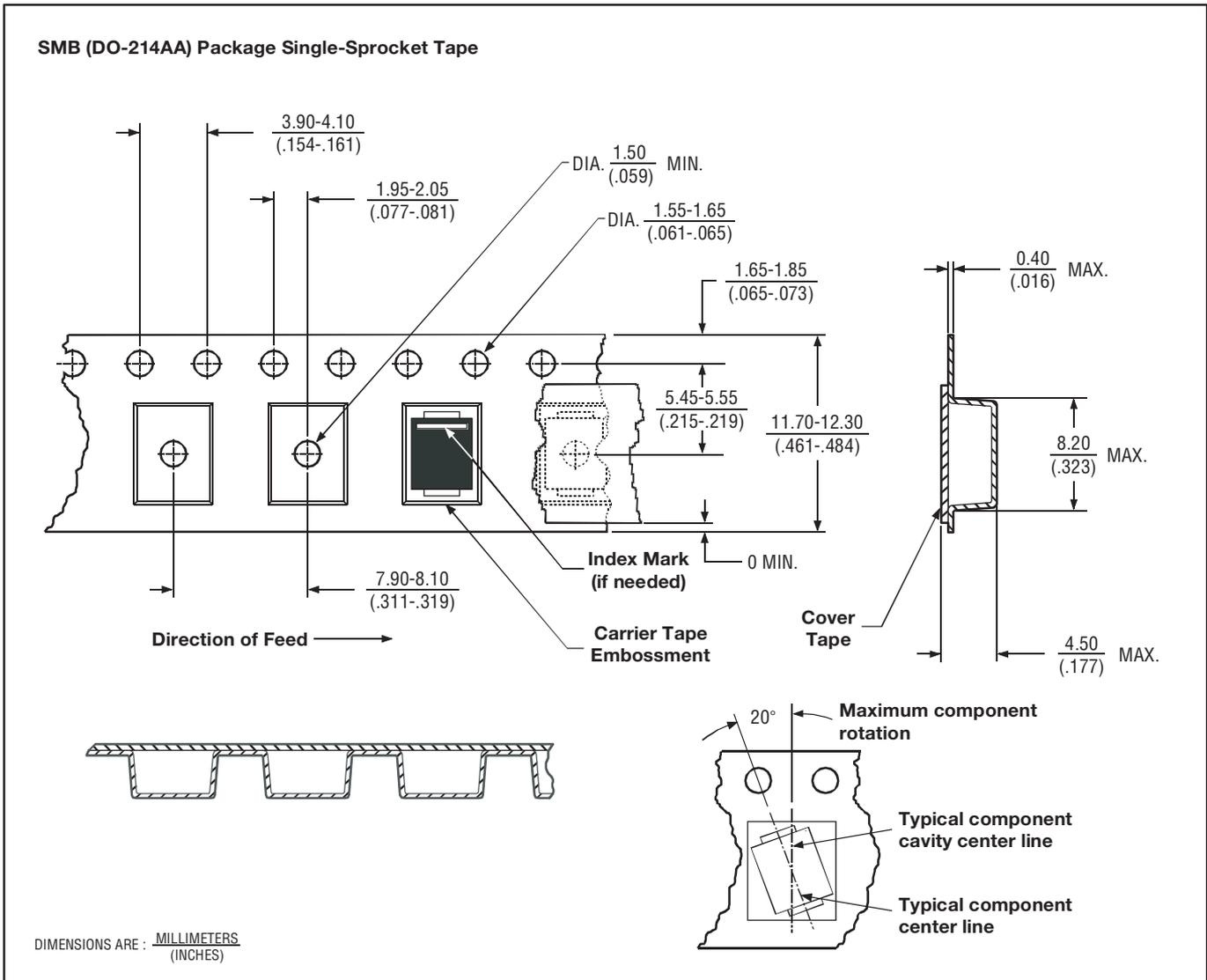
NOTES: A. The clearance between the component and the cavity must be within 0.05 mm (.002 in) MIN. to 0.65 mm (.026 in) MAX. so that the component cannot rotate more than  $20^\circ$  within the determined cavity.
