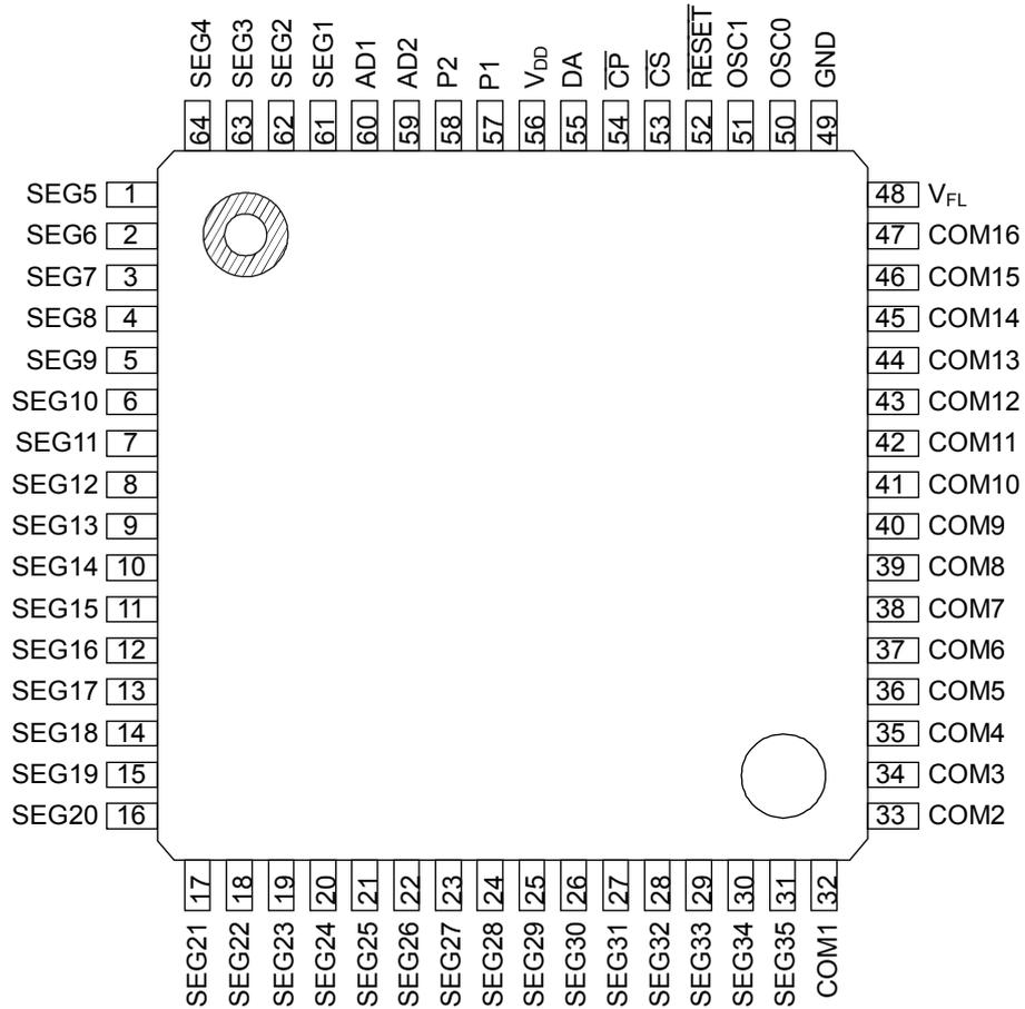
**64-Pin Plastic QFP / TQFP**
