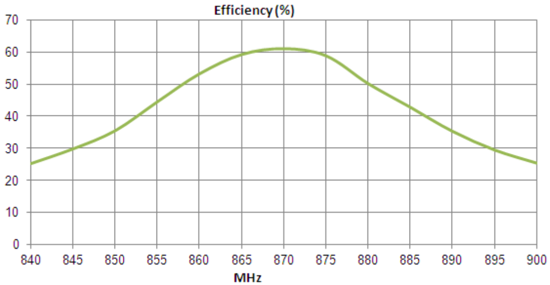
Figure 4. Efficiency of 868 MHz ISM Band Antenna ILA.02
