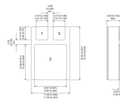
Bipolar PNP Device in a Hermetically sealed **Ceramic Surface Mount** Package for High **Reliability Applications**
