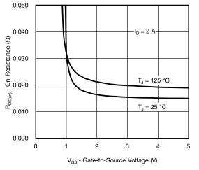
On-Resistance vs. Gate-to-Source Voltage
