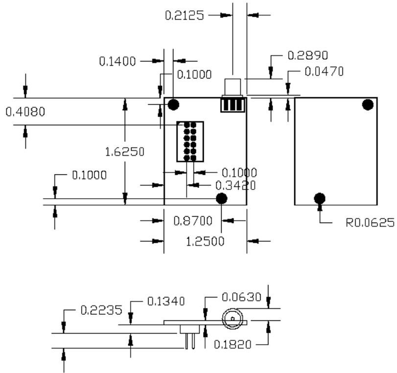
Figure 5-1: Mechanical Dimensions (all measures are in inches)
