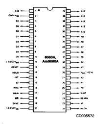
Note: Pin 1 is marked for orientation
