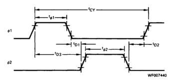
$t_{CY} = t_{D3} + t_{r\phi2} + t_{\phi2} + t_{f\phi2} + t_{D2} + t_{r\phi1}$
