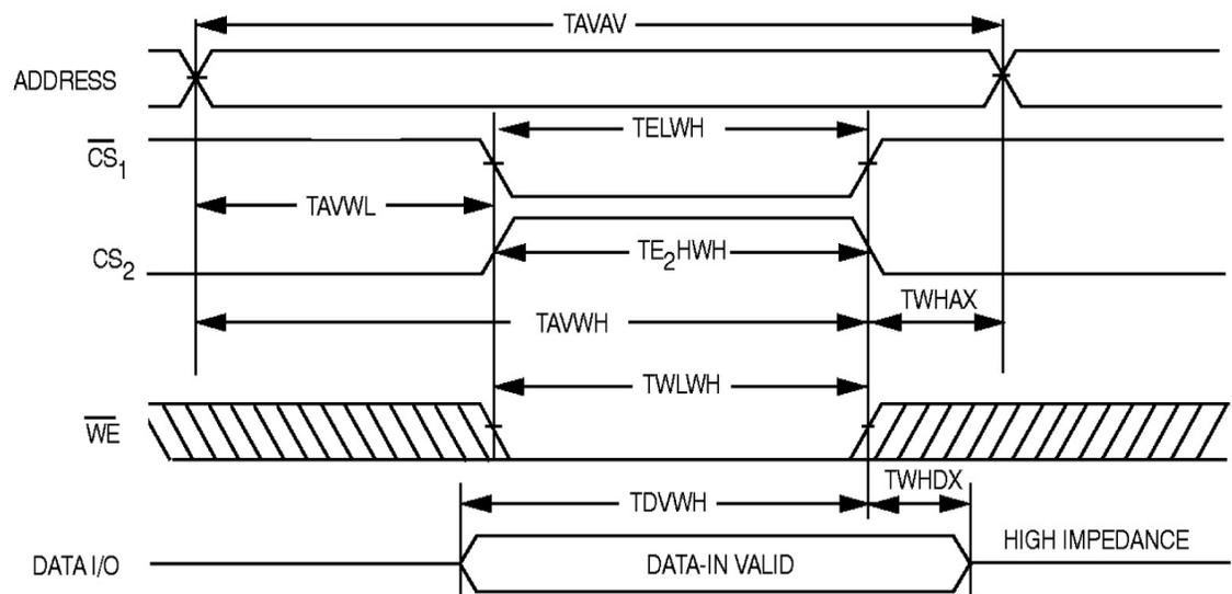
Note: The internal write time of the memory is defined by the overlap of  $\overline{CS1}$  Low and CS2 HIGH and  $\overline{WE}$  LOW. Both signals must be activated to initiate a write and either signal can terminate a write by going in active. The data input setup and hold timing should be referenced to the activated edge of the signal that terminates the write. Data out is high impedance if  $OE = V_{IH}$ .
