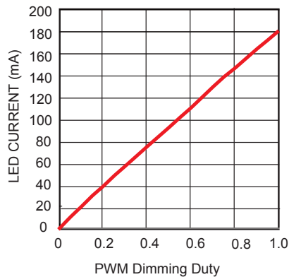
LED Current vs. PWM Dimming Duty
