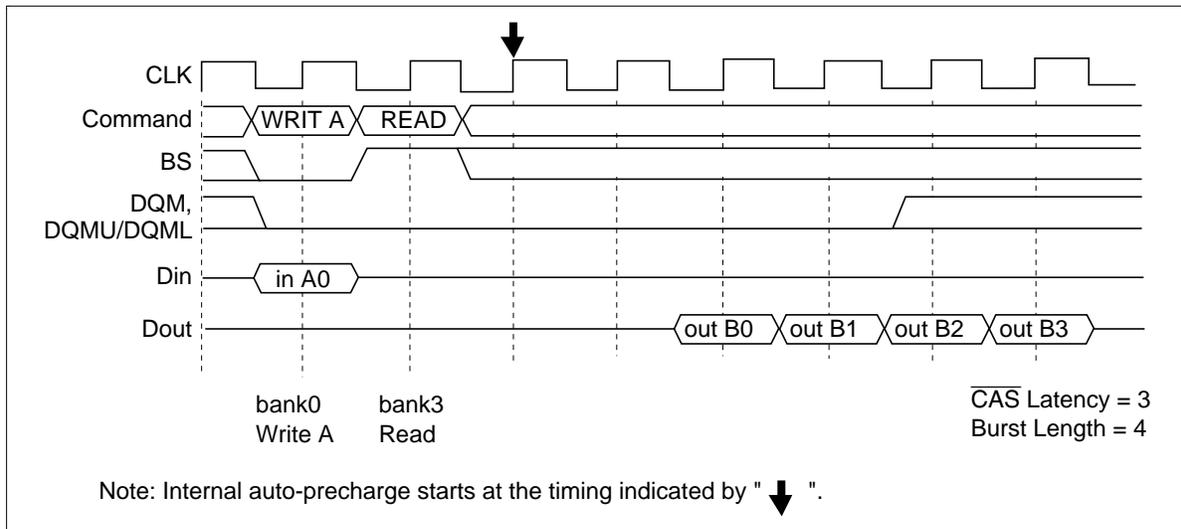
**2. Same bank:** The consecutive read command from write with auto precharge (the same bank) is illegal. It is necessary to separate the two commands with a bank active command.
