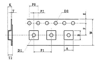
\* The dimensions of A and B are reference values the following information's for the component.
