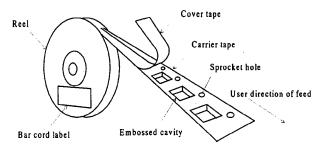
The embossed taping are inserted a component into the carrier tape and pasted the cover tape on the upper side. The reel flange has a gauge for remaining components roughly.
