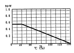
Approximate power dissipation Pd  $\neq$  600mW at 25°C / derating value 4.8mW/°C /  $\theta$  ja = 208°C/W
