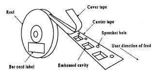
The embossed taping are inserted a component into the carrier tape and pasted the cover tape on the upper side. The reel flange has a gauge for remaining components roughly.
