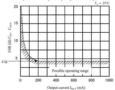
Output current vs. Input / Output capacitor ESR (equivalent series resistance)
