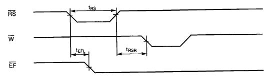
**NOTES:** 1.  $\overline{W} = \overline{R} = V_{IH}$  during reset.
