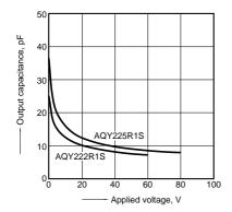
12.-(2) Output capacitance vs. applied voltage characteristics
