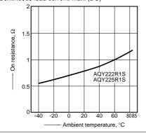
2.-(2) On resistance vs. ambient temperature characteristics
