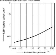
LED turn off current vs. ambient temperature characteristics
