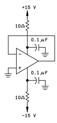
FIGURE 2. Radiation exposure circuit.
