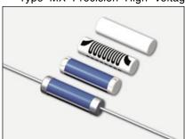
Inductive serpentine pattern with a patented, high thru-put screen printed silicone coating. The alignment of the gap in the coating pattern with the gap in the serpentine resistor pattern provides a complete encapsulation of the resistor element. The cap and lead assemblies are pressed onto the resistor core, finishing the resistor and providing rugged terminal attachment.
