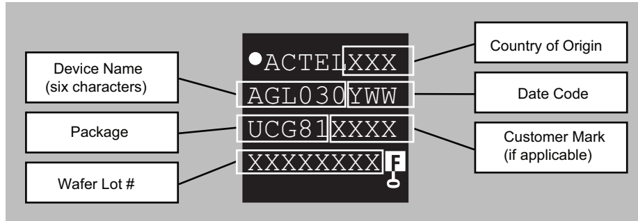
Figure 1 • Example of Device Marking for Small Form Factor Packages
