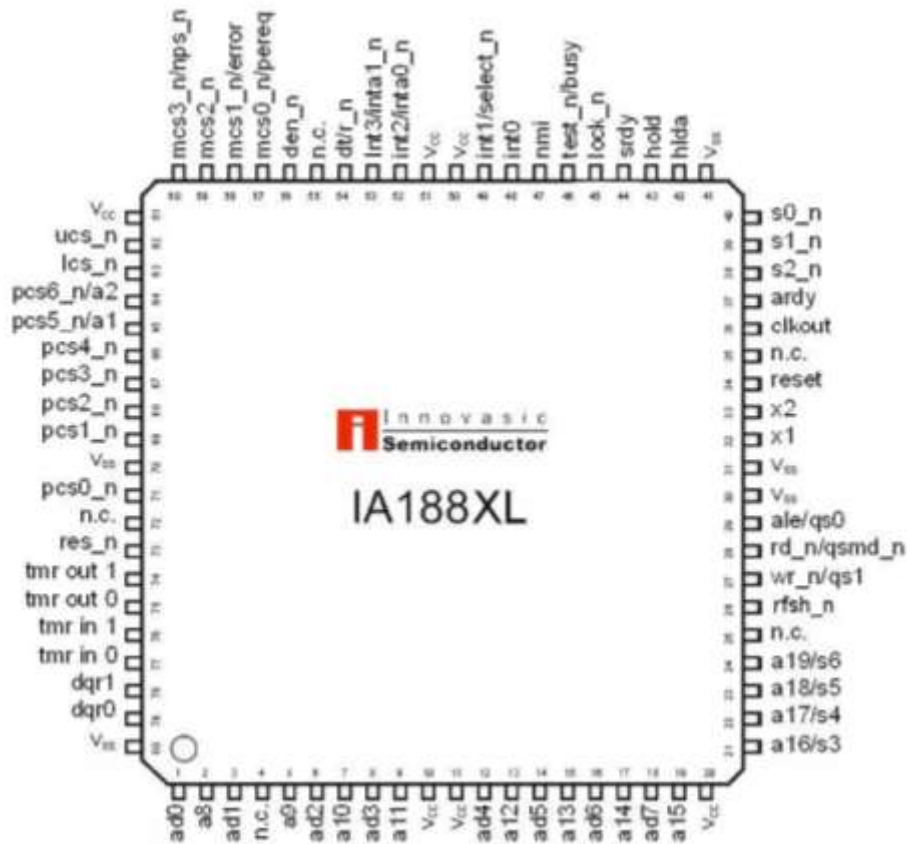
Figure 8. IA188XL 80-Lead LQFP Package Diagram
