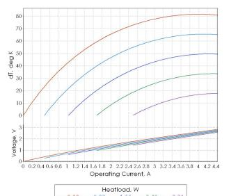
**Note**: Performance data is specified at optimal conditions (TEC hot side is stabilized at ambient temperature). Heatsink thermal resistance is not included into estimations. Use TECCad Software for estimations under different conditions.
