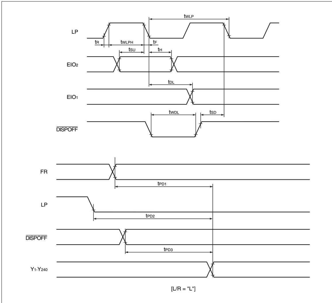
( $V_{SS} = V_5 = 0$  V,  $V_{DD} = +2.5$  to  $+5.5$  V,  $V_0 = +15.0$  to  $+42.0$  V,  $T_{OPR} = -20$  to  $+85$  °C)
