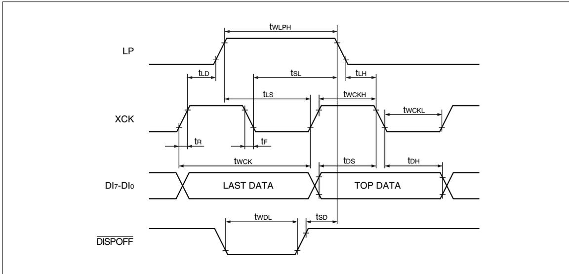
( $V_{SS} = V_5 = 0 \text{ V}$ ,  $V_{DD} = +5.0 \pm 0.5 \text{ V}$ ,  $V_0 = +15.0 \text{ to } +42.0 \text{ V}$ ,  $T_{OPR} = -20 \text{ to } +85 \text{ }^\circ\text{C}$ )
