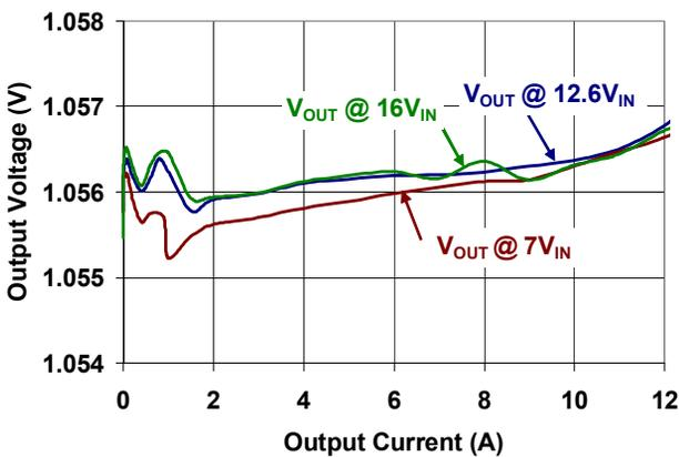
Figure 5. Output Voltage Regulation vs. Output Current
