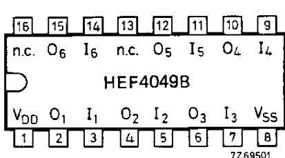
Fig.2 Pinning diagram.
