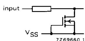
Fig.4 Input protection circuit that allows input voltages in excess of V<sub>DD</sub>.**FAMILY DATA, I<sub>DD</sub> LIMITS category BUFFERS**
