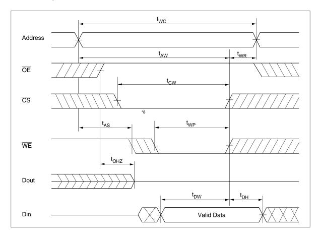
Write Timing Waveform (2)  $(\overline{OE} Low Fixed)$
