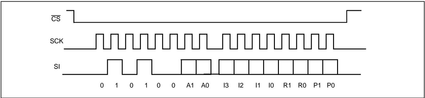
Figure 4. Three-Byte Command Sequence (Write)
