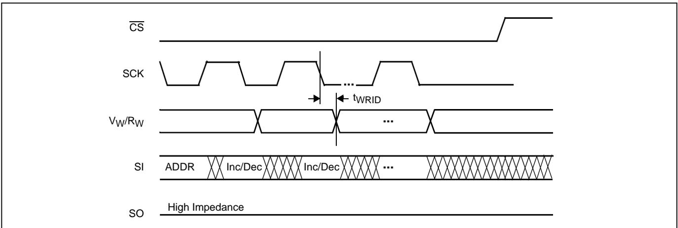
Write Protect and Device Address Pins Timing
