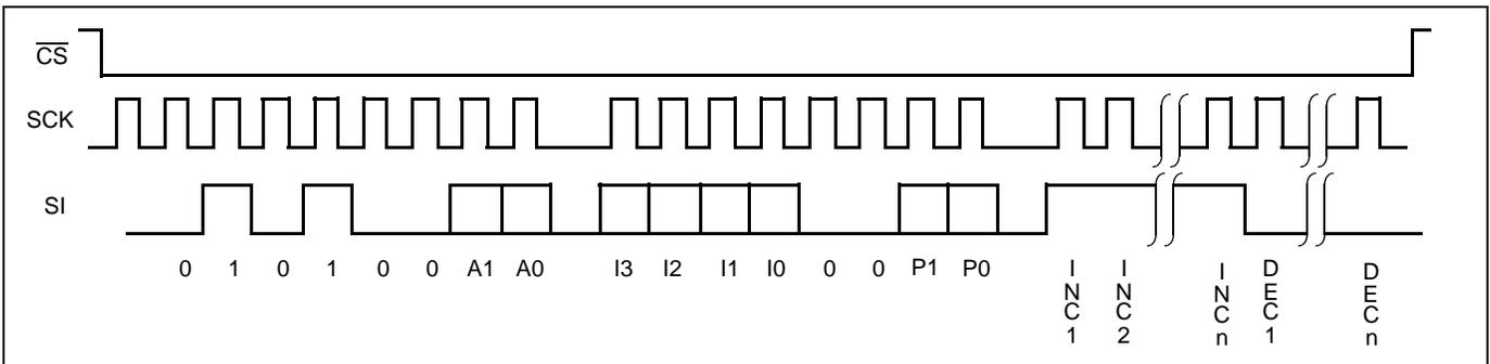
Figure 7. Increment/Decrement Timing Limits
