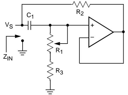
$Z_{IN} = R_2 + s R_2 (R_1 + R_3) C_1 = R_2 + s L_{eq}$
