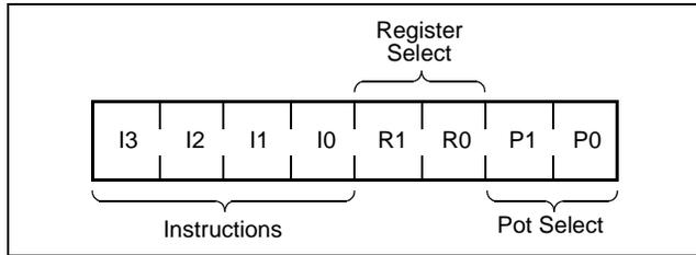
The four high order bits of the instruction byte specify the operation. The next two bits ( $R_1$  and  $R_0$ ) select one of the four registers that is to be acted upon when a register oriented instruction is issued. The last two bits ( $P_1$  and  $P_0$ ) selects which one of the four potentiometers is to be affected by the instruction.
