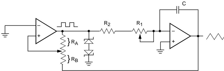
frequency  $\propto R_1, R_2, C$
