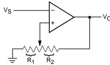
$$V_{UL} = \{R_1 / (R_1 + R_2)\} V_O(\text{max})$$
