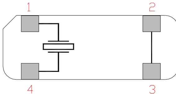
**Pin 2 & 3 connected to metal case**
