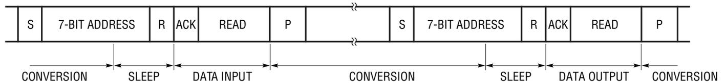
**Figure 5. Consecutive Reading with the Same Input/Configuration**
