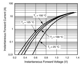
Fig. 3 - Typical Instantaneous Forward Characteristics
