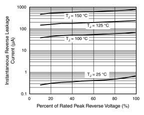
Fig. 4 - Typical Reverse Leakage Characteristics
