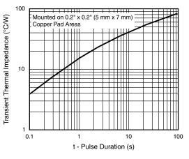
Fig. 6 - Typical Thermal Impedance
