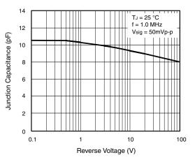
Fig. 5 - Typical Junction Capacitance
