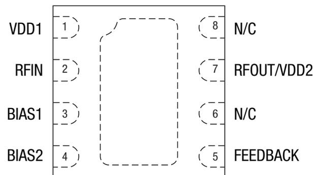
**Figure 2. SKY65037-360LF Pinout – 8-Pin QFN (Top View)**
