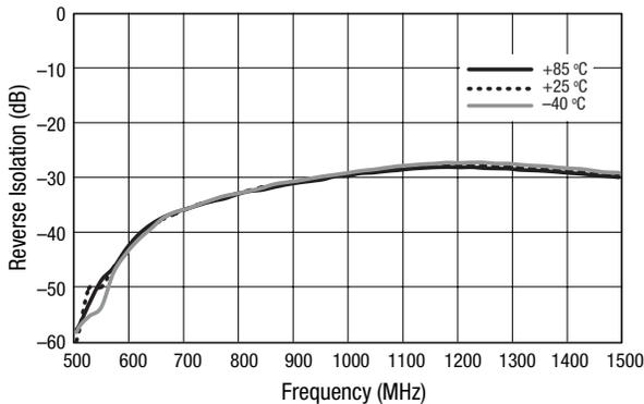
Figure 7. Reverse Isolation vs Frequency Over Temperature, PIN = -20 dBm
