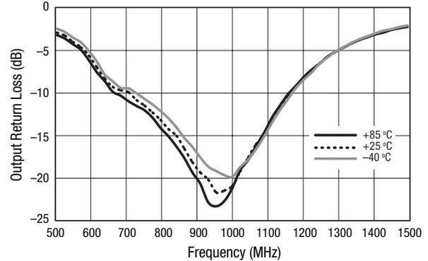
Figure 4. Output Return Loss vs Frequency Over Temperature, PIN = -20 dBm
