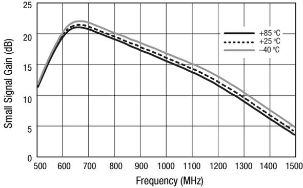
Figure 3. Small Signal Gain vs Frequency Over Temperature, PIN = -20 dBm
