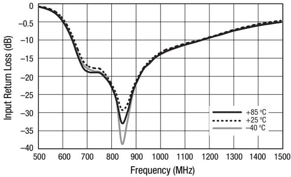
Figure 5. Input Return Loss vs Frequency Over Temperature, PIN = -20 dBm
