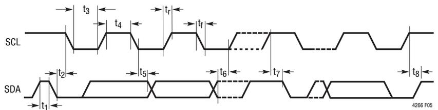
Figure 5. I<sup>2</sup>C Interface Timing
