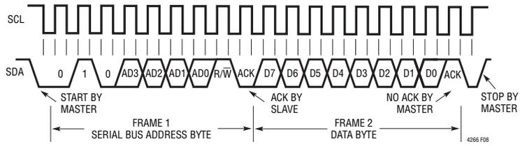
Figure 8. Reading the Interrupt Register (Short Form)
