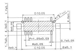
Note 1.If the pattern exists in the shaded area, and isn't treated with resist, it could touch the connector contact.
