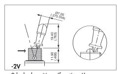
2 locked positions (function 6) Typical angle of throw : 26°
