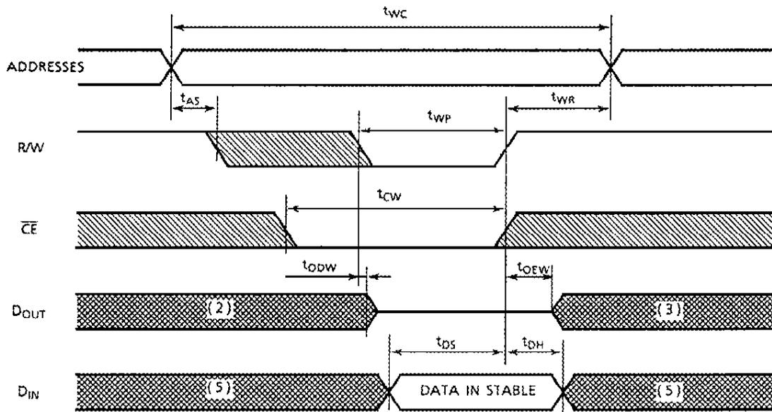
Write Cycle 2 <sup>(4)</sup> ( $\overline{CE}$  Controlled Write)
