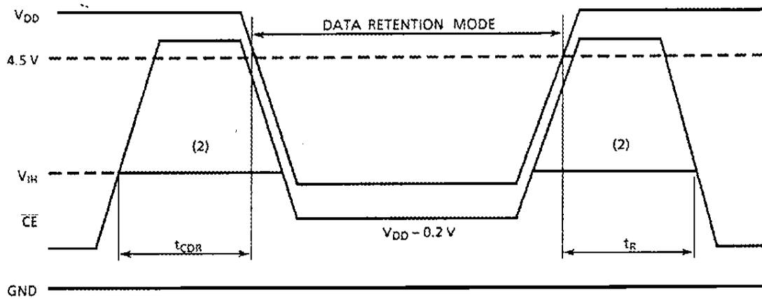
Note (2): If the V<sub>IH</sub> of  $\overline{CE}$  is 2.2V in operation, I<sub>DD2</sub> current flows during the period that the V<sub>DD</sub> voltage is going down from 4.5V to 2.4V.
