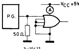
INPUT WAVEFORM IS THE SAME AS THAT IN CASE OF SWITCHING CHARACTERISTICS TEST
