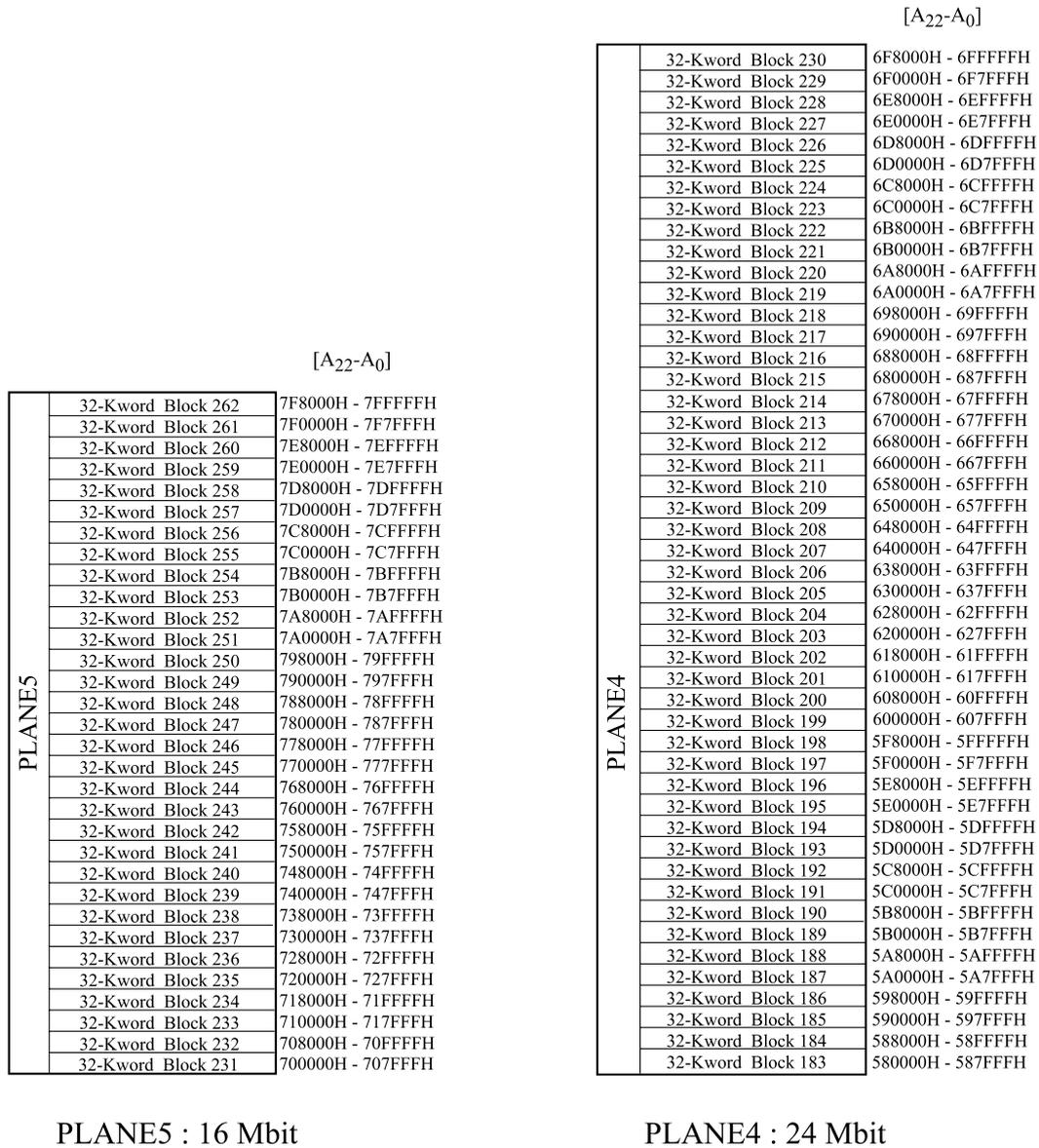
Figure 2.3. Memory Map (Bottom Parameter, Plane 4 and Plane 5)
