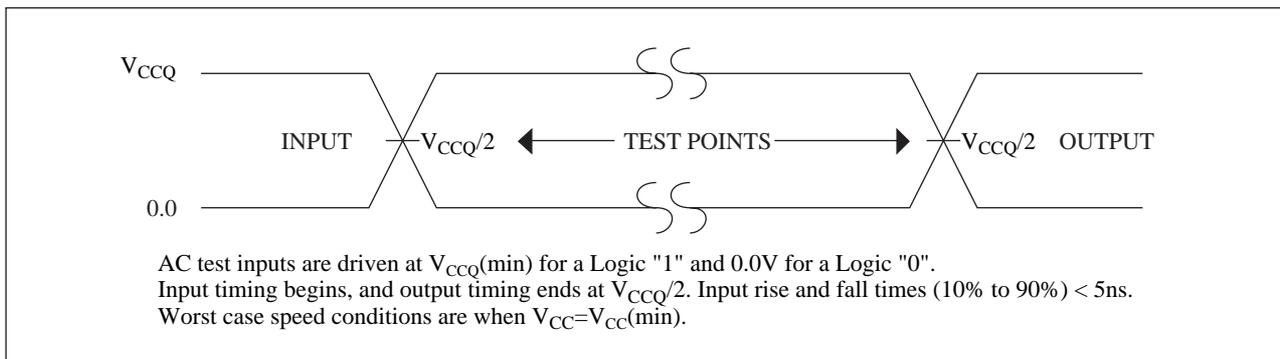
Figure 4. Transient Input/Output Reference Waveform for  $V_{CC}=2.7\text{V}-3.3\text{V}$
