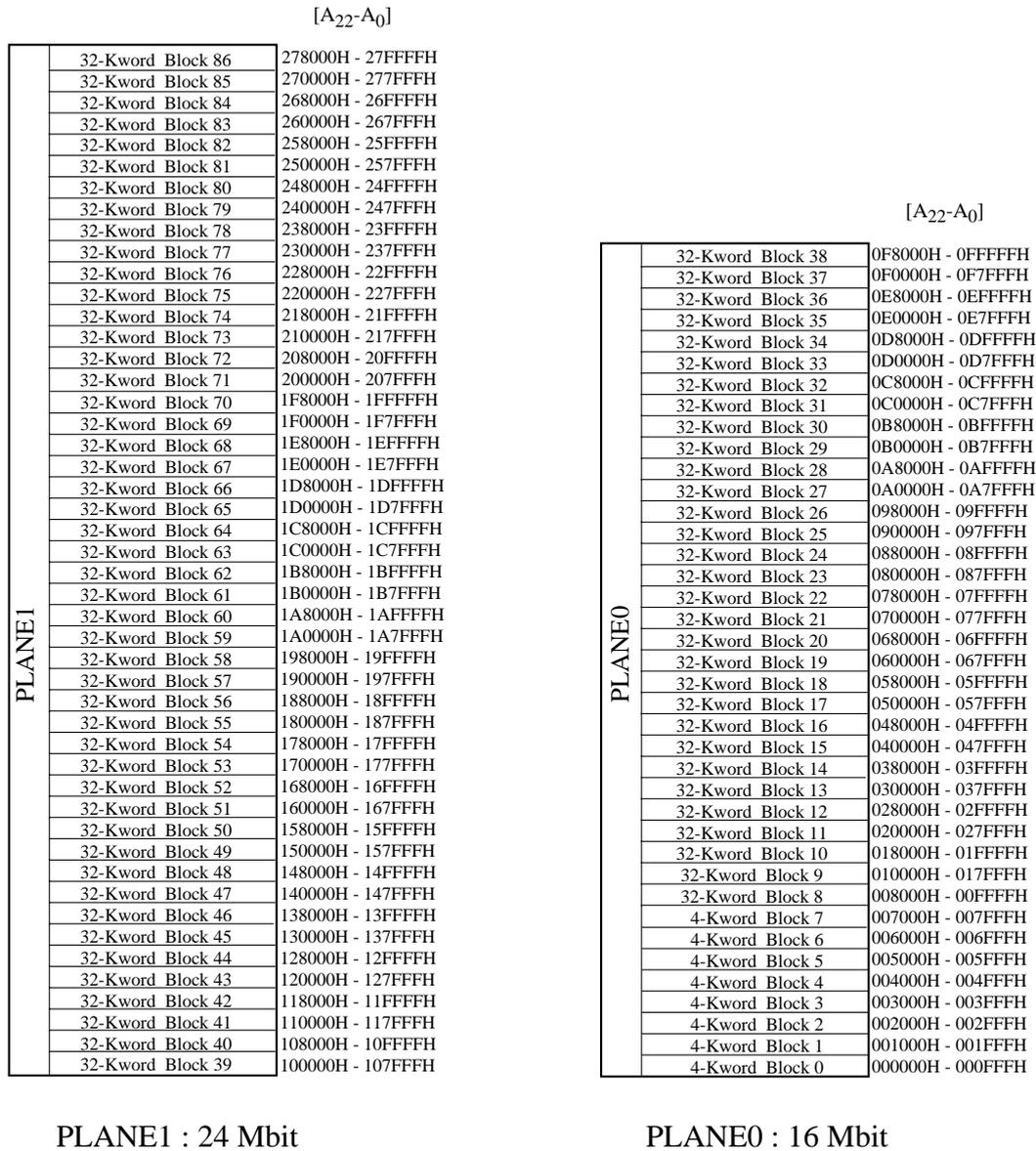
Figure 2.1. Memory Map (Bottom Parameter, Plane 0 and Plane 1)
