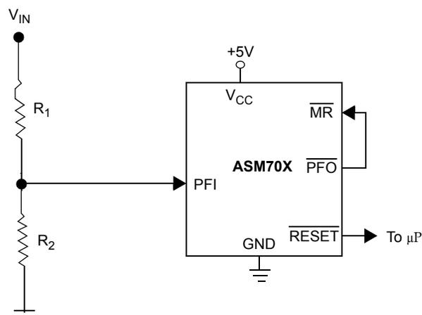
Figure 4: Monitoring +5V and an additional supply V<sub>IN</sub>
