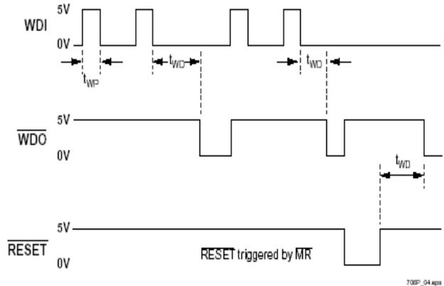
Figure 1: WDI Three-state operation
