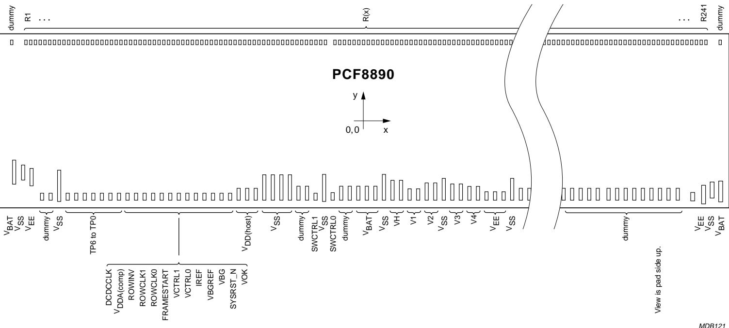
Fig.11 Bonding pad location.
