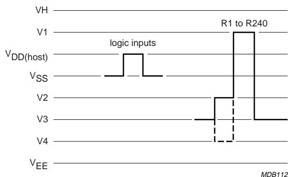
Fig.2 I/O signal voltage levels.
