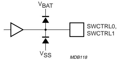
Fig.8 Switching control outputs.
