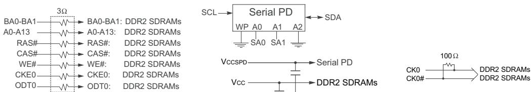
NOTE: All resistor value, are 22 ohms ± 5% unless otherwise specified.
