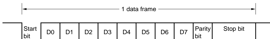
Figure 14-10: Format of Transmit/Receive Data in Asynchronous Serial Interface
