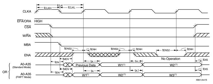
Figure 14. Port-A Read Cycle Timing for FIFO2 (IDT Standard and FWFT Modes)
