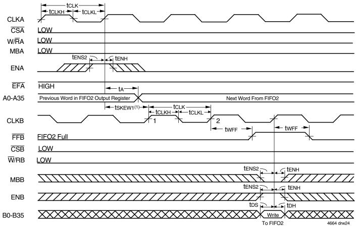
Figure 22. FFB Flag Timing and First Available Write when FIFO2 is Full (IDT Standard Mode)
