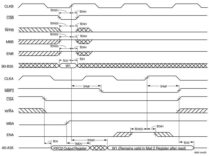
Figure 28. Timing for Mail2 Register and MBF2 Flag (IDT Standard and FWFT Modes)
