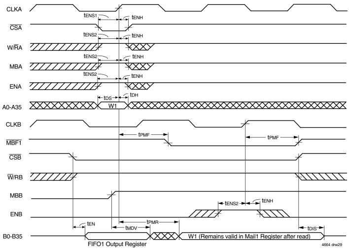
Figure 27. Timing for Mail1 Register and MBF1 Flag (IDT Standard and FWFT Modes)
