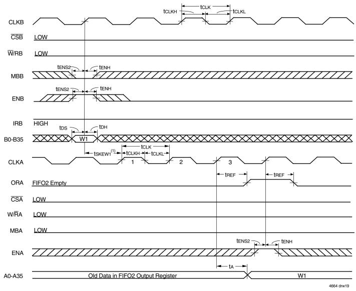
Figure 17. ORA Flag Timing and First Data Word Fall through when FIFO2 is Empty (FWFT Mode)
