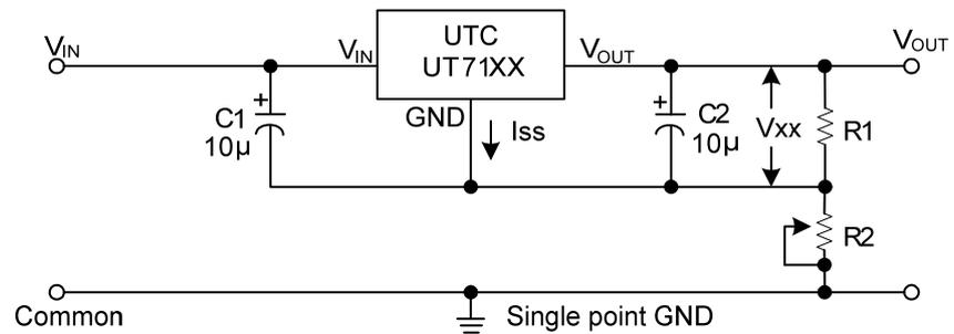
$$V_{OUT} = V_{XX} \left(1 + \frac{R_2}{R_1}\right) + I_{SS} R_2$$
