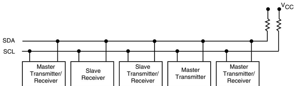
Note: Due to open drain configuration of SDA, a bus-level resistor is called for (Typical value = 4.7Ω)
