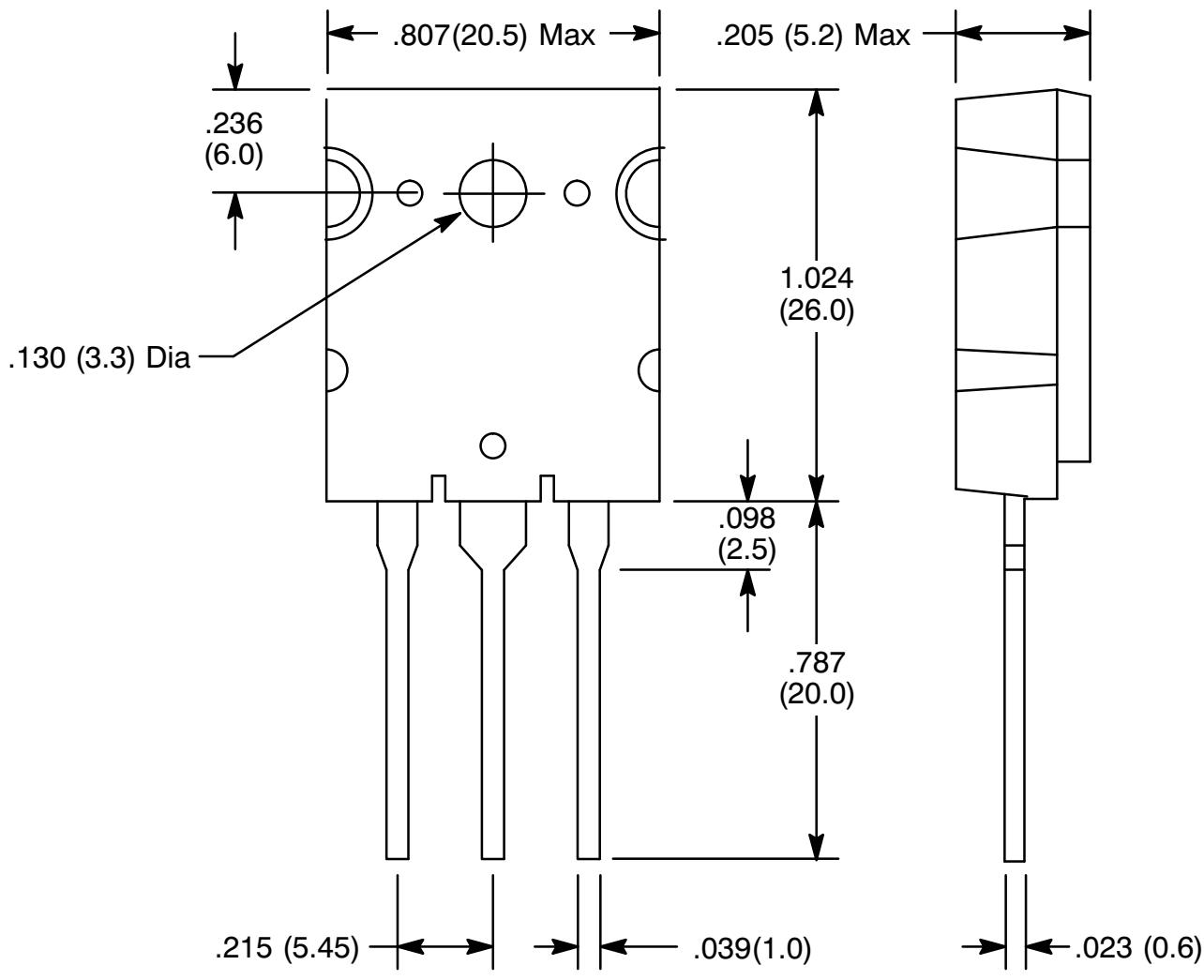
**Note:** Pin2 connected to heat sink
