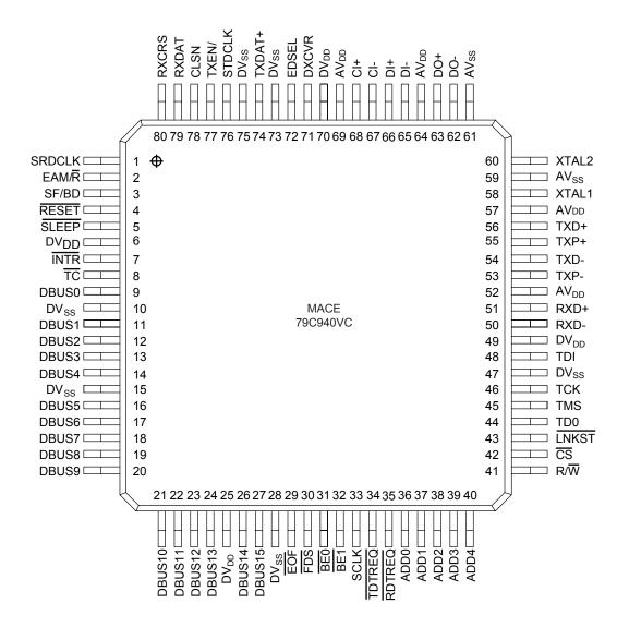
**Notes:** Four pin functions available on the PLCC and PQFP packages are not available with the TQFP package. (See full data sheet for description of pins not included with the 80-pin TQFP package. In particular, see section "Pin Functions not available with the 80-pin TQFP package.")
