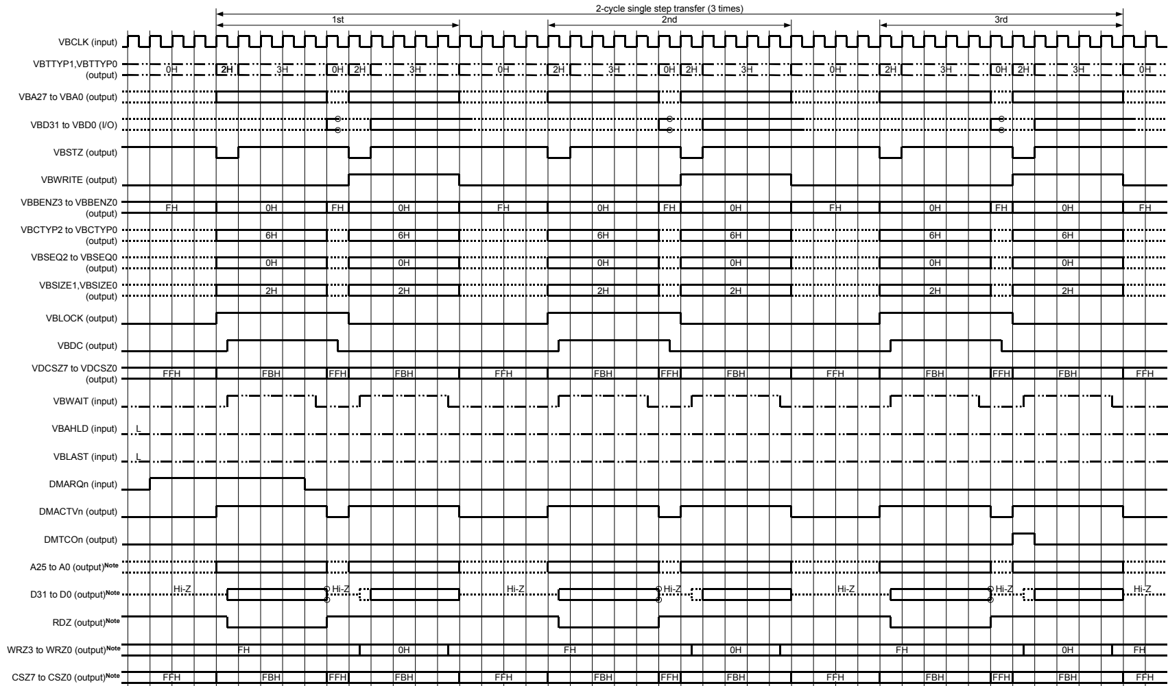
Figure 7-28. Example of Two-Cycle Single-Step Transfer Timing (Between External SRAMs Connected to NB85E500)
