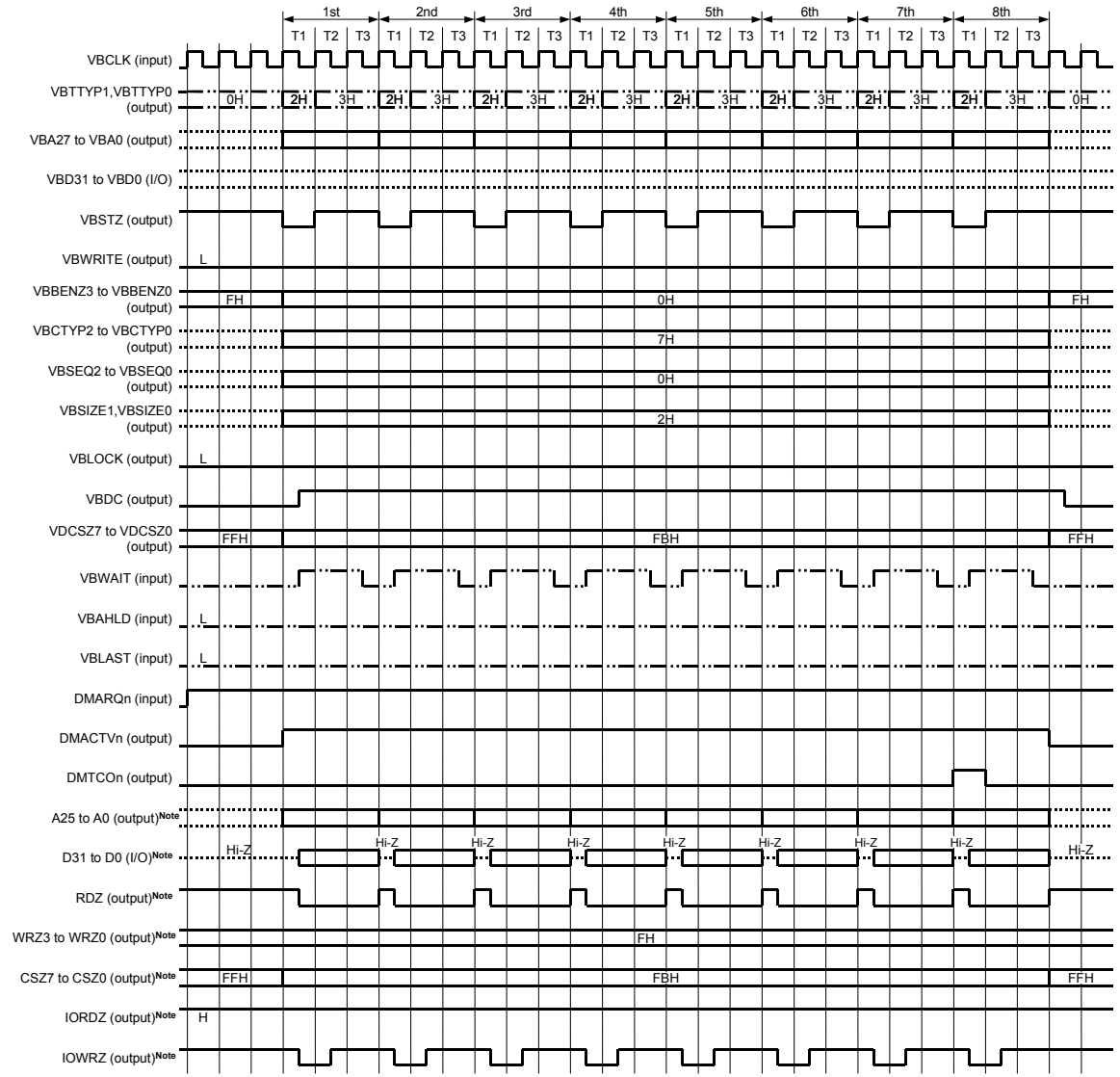
Figure 7-37. Example of Flyby Block Transfer Timing (from External SRAM to External I/O Connected to NB85E500)
