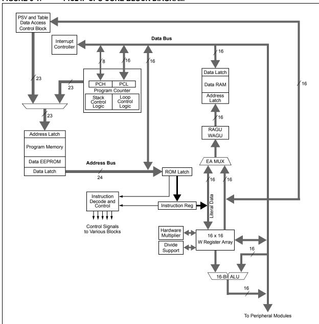
FIGURE 3-1: PIC24F CPU CORE BLOCK DIAGRAM
