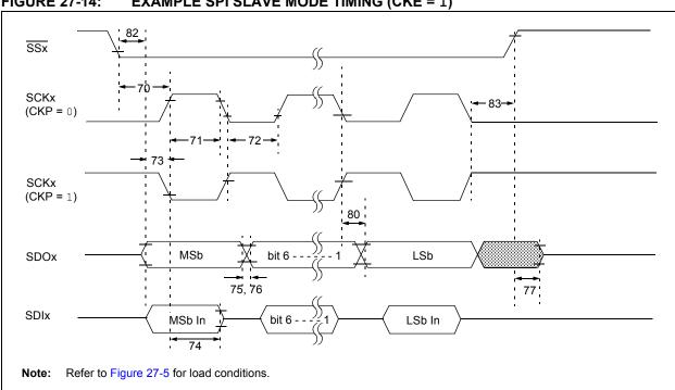
FIGURE 27-14: **EXAMPLE SPI SLAVE MODE TIMING (CKE = 1)**
