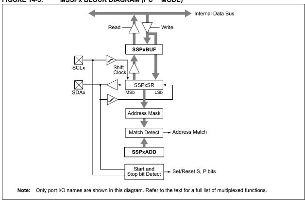
FIGURE 14-4: MSSPx BLOCK DIAGRAM (I<sup>2</sup>C™ MASTER MODE)
