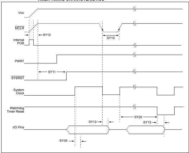
FIGURE 27-9: BROWN-OUT RESET CHARACTERISTICS
