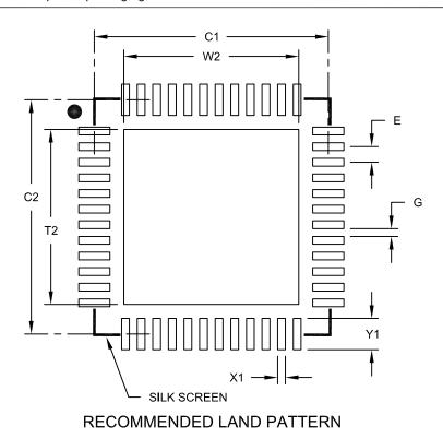
Units **MILLIMETERS Dimension Limits** MIN NOM MAX Contact Pitch Ε 0.40 BSC Optional Center Pad Width W2 4.45 Optional Center Pad Length T2 4.45 Contact Pad Spacing C1 6.00 Contact Pad Spacing C2 6.00 Contact Pad Width (X28) X1 0.20 Contact Pad Length (X28) <u>Y1</u> 0.80 Distance Between Pads G 0.20
