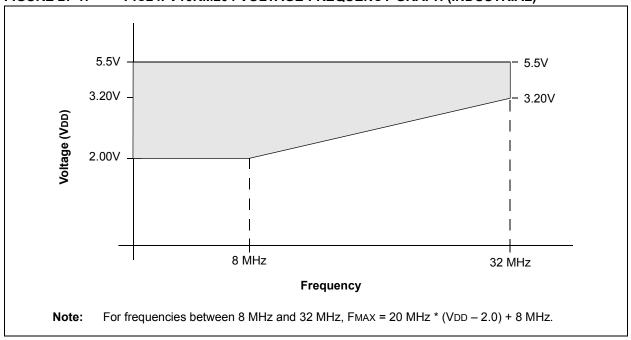
FIGURE 27-2: PIC24F16KM204 FAMILY VOLTAGE-FREQUENCY GRAPH (INDUSTRIAL)
