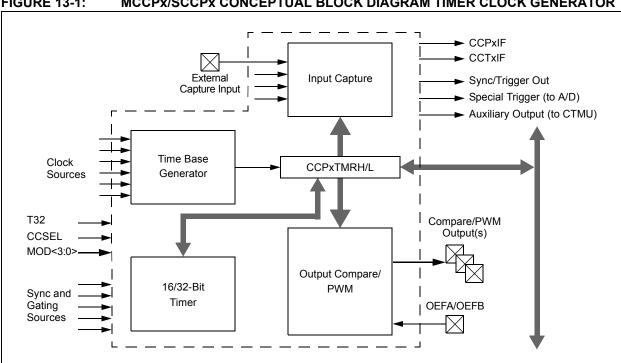
**FIGURE 13-1:** MCCPx/SCCPx CONCEPTUAL BLOCK DIAGRAM TIMER CLOCK GENERATOR
