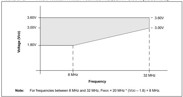
FIGURE 27-3: PIC24FV16KM204 VOLTAGE-FREQUENCY GRAPH (EXTENDED)
