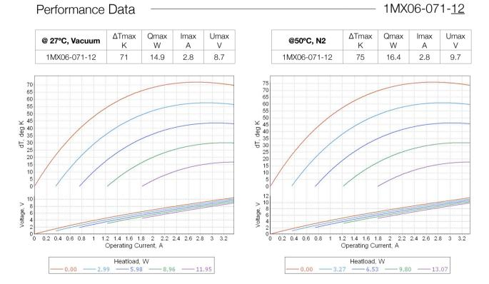
**Note**: Performance data is specified for optimal optimal conditions (TEC hot side is stabilized at ambient temperature). Heatsink thermal resistance is not included into estimations. Use TECCad Software for estimations under different conditions.
