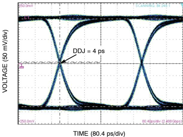
**Figure 7. Typical Output Waveform at 2.488 Gb/s with PRBS 2<sup>23</sup>-1 (Input Signal DDJ = 12 ps)**
