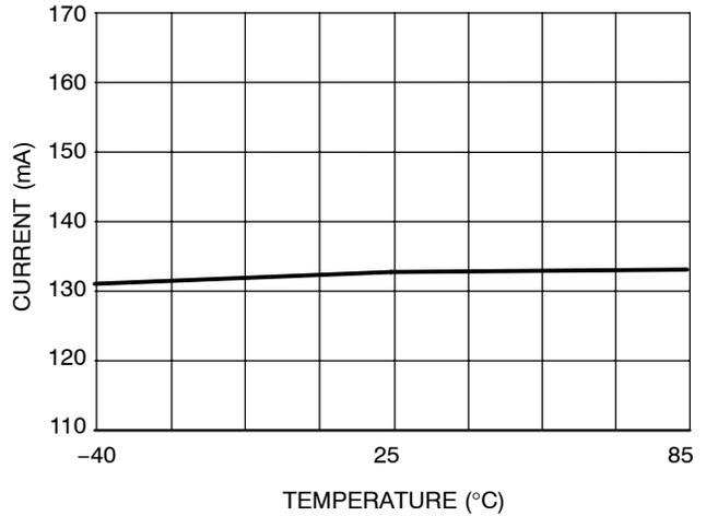
**Figure 6. Supply Current vs. Temperature (All 4 Outputs Enabled)**
